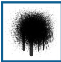
Too much paint produces these drippings
